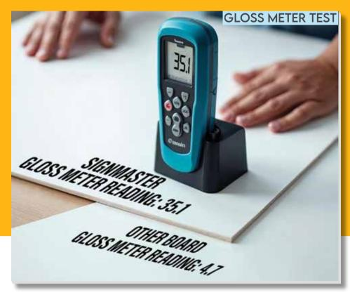
\*A Gloss Meter is an instrument that measures how much light reflects off a surface. It helps ensure your prints have the perfect finish. A higher gloss level means sharper images, richer colours, and a professional look that stands out.
